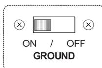
Your amplifier has a mains socket outlet with a ground connection. The use of this type of connection is recommended for electrical safety reasons (including wetlands). However sometimes this connection «mass» is the origin of «hum» audible from the speakers in a hi-fi system to solve this problem, the cancellation of the ground connection is sometimes sufficient. To do this you have, under the device, a switch to choose to connect or not the mass of the device to the mains.
