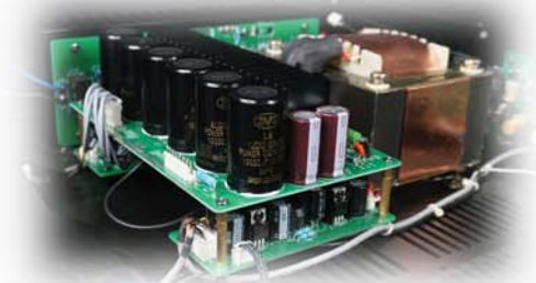
Power supply with Capacitors and Transformer
